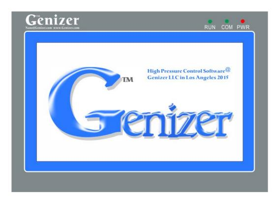
2) The display of the touch screen has three indicator lights on its top right corner. From left to right the three indicator lights are: RUN, the PLC indicator light; COM, the communication light; PWR, the power indicator light of the touch screen. Then machine is ready when all the lights are lit on. Otherwise, inspection is needed and the equipment cannot be started until the malfunction is resolved.
